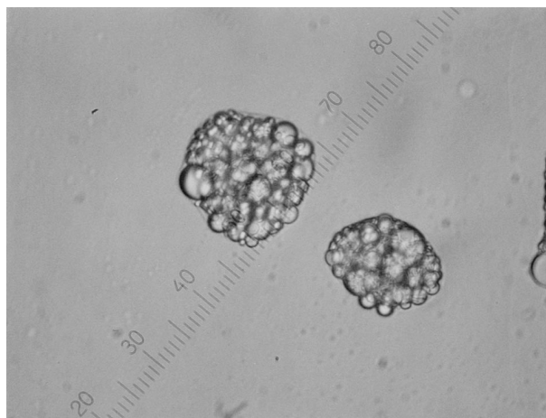
Figure 7. Gelled microcapsules with oily core (optical microscope).
